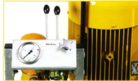
Control panel WS-400 H at HAG-12.2
